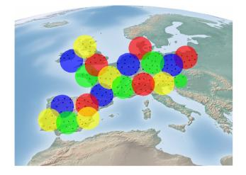
Figure 8: Example of beam layout solution with only circles as beam shape
