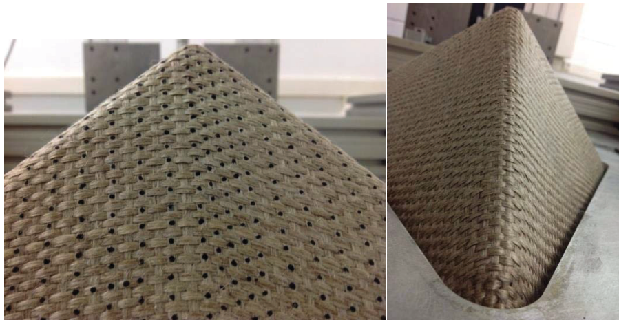
FIGURE 8 : Un-balanced plain weave fabric without tow buckles
