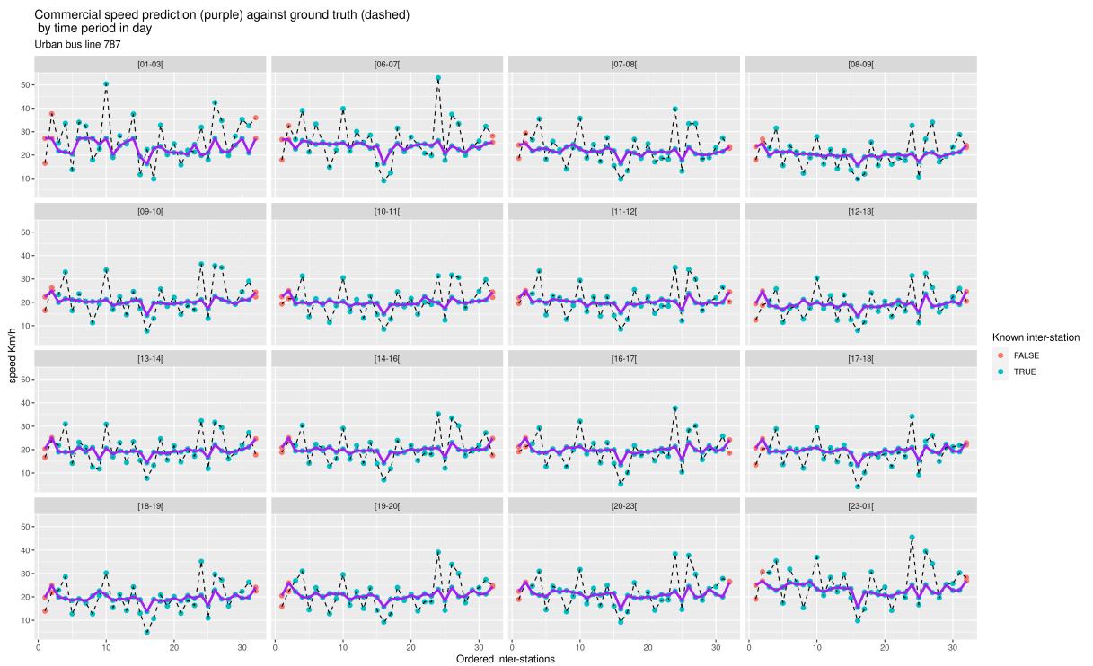
Figure A.4 – micro-predictions of bus line 787 with and without OSM features
