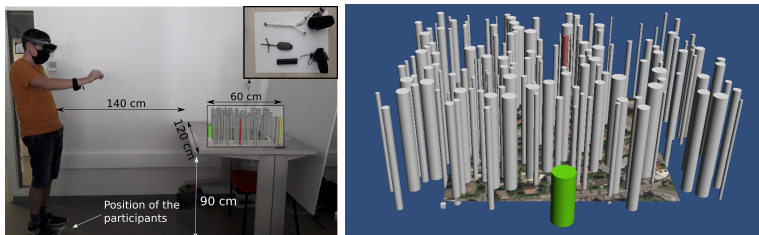
Fig. 4: Setup of the experiment (left) and example of a 3D scene (right) with a start target in green, a goal target in red and distractors in grey.
