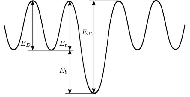
Figure 1: Energy diagram presenting diffusion energy  $E_D$ , trapping energy  $E_t$ , binding energy  $E_b$  and detrapping energy  $E_{dt}$ . This diagram illustrates the assumption that  $E_D = E_t$  and explicits the relation between trapping, detrapping and diffusion :  $E_{dt} = E_D + E_b$
