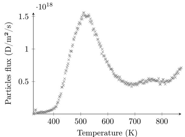
Figure 6: Thermal desorption spectrometry spectrum of deuterium in Eurofer97. The sample was loaded under deuterium atmosphere of  $9 \cdot 10^4$  Pa at 673 K for 6 hours. TDS was then performed with a 1 K/s temperature ramp-up.
