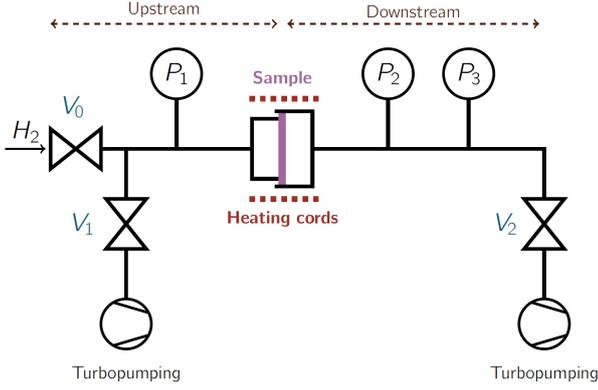
Figure 2: Diagram presenting the Hypertomate hydrogen permeation experiment
