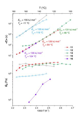
**Fig. 5** Temperature dependence of top) the average relaxation times and bottom) zero-shear moduli for TPIL dynamic networks **11** (red solid circles), **12** (blue open triangles), **14** (green solid triangles). Additional data for previously reported aliphatic TPIL dynamic network **15** (black open squares) and polystyrene-based TPIL dynamic network **16** (purple solid diamonds) have been added for comparison.<sup>21,41</sup>.
