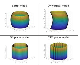
Figure 2. Illustration of some of the considered modes in the chosen basis description (amplitudes have been enhanced for more visibility)
