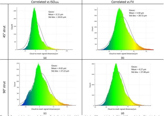
Figure 5. Computed cloud-to-mesh distances for both struts: (a) and (c) correlated vs ISO<sub>50%</sub> point clouds; (b) and (d) correlated vs FV point cloud
