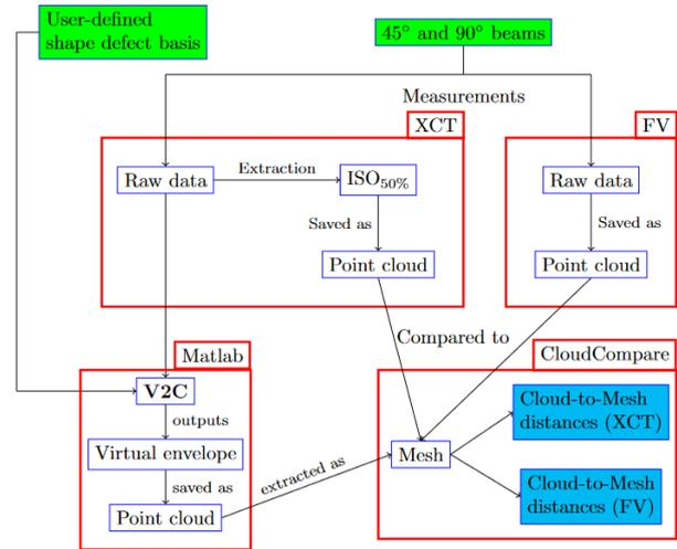
Figure 4. Data processing pipeline. Inputs are filled in green and outputs are filled in blue.
