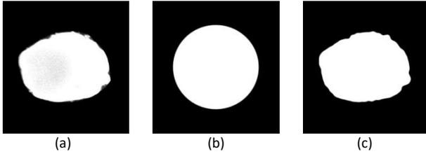
Figure 1. Illustration of V2C on a 2D strut cross-section: (a) XCT physical measurement; (b) initial virtual shape; (c) computed virtual shape defect
