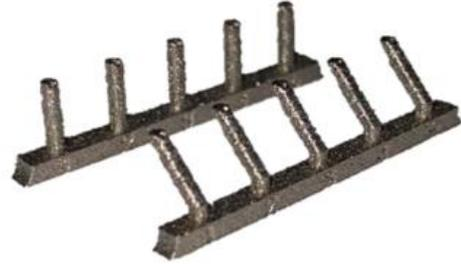
Figure 3. Vertical and inclined BCCz representative printed struts. (One strut from each set has been considered in the following)
