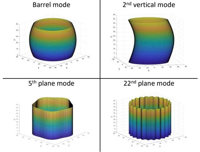
Figure 2. Illustration of some of the considered modes in the chosen basis description (amplitudes have been enhanced for more visibility)
