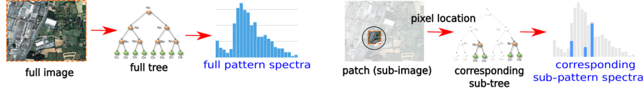
Fig. 4: (Left) Pattern spectra is a histogram-like distribution of image components. (Right) The components of each image patch contribute to a few numbers of histogram bins creating a sub-pattern spectra.
