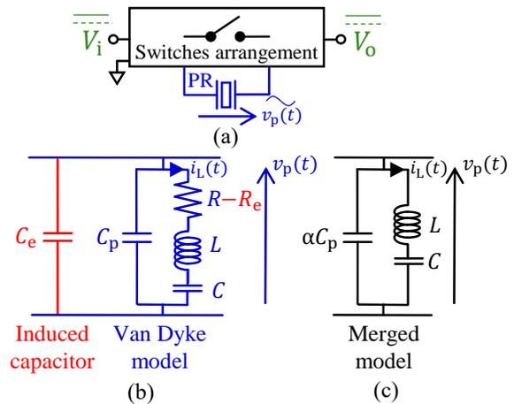
Fig. 1. (a) PR DC-DC converter, (b) electrically induced capacitor, and (c) merged model.
