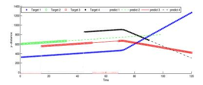
Figure 4: y-direction evolutions over time of 4 targets.
