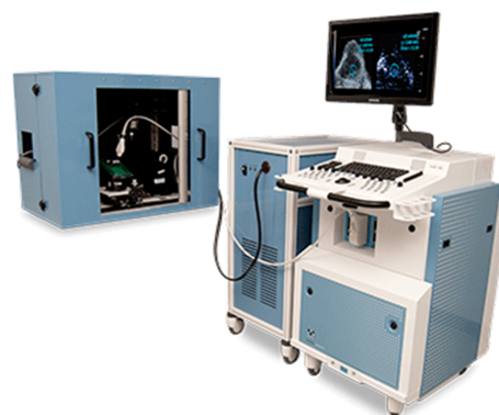
Figure 2. Commercial multispectral photoacoustic system: Vevo LAZR.
