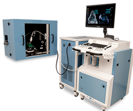
Figure 2. Commercial multispectral photoacoustic system: Vevo LAZR.
