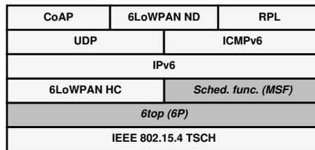
Fig. 2: Network stack in the 6TiSCH architecture.
