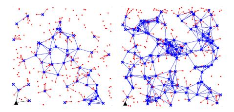
**Fig. 1.** Two networks obtained for fixed drones' positions, randomly chosen. Parameter values:  $r_{p2d} = 80, L = 1000$  and  $r_{2d2} = 150$ . On the left side n = 50 and n = 120 on the right side. Crosses are drones, points are people, the antenna is represented by a black triangle at the bottom left corner of the area.
