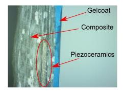
Figure 3: Close-up view of a smart material slice
