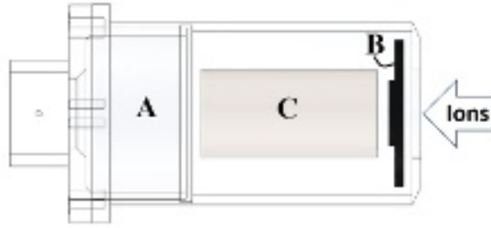
FIG. 4. Main parts of a Faraday cup
