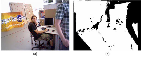
Figure 7: (a) Static features points after eliminating the dynamic feature points. (b) Mask generated using Optical Flow and Initial Camera motion estimation which depicts the dynamic objects in black and static objects in white.
