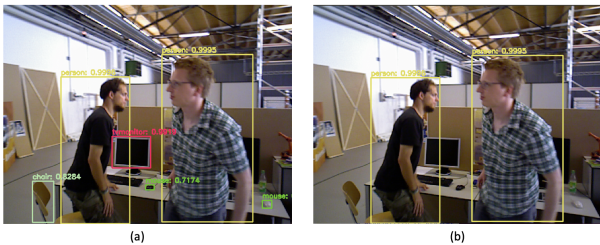
Figure 2: (a) Object detection using YOLO. (b) Potential dynamic object detection.
