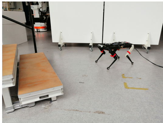
Fig. 1: Experimental setup: a RealSense D435i is mounted on the Solo robot which localizes itself with respect to stairs. A motion capture system provides ground truth of the robot pose.
