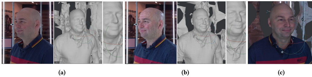
Figure 8: (a) Geometry and texturing estimated without (b) and with light pattern projection; (c) Geometry estimated with light pattern projection and texturing estimated without light pattern (dataset from [49]).
