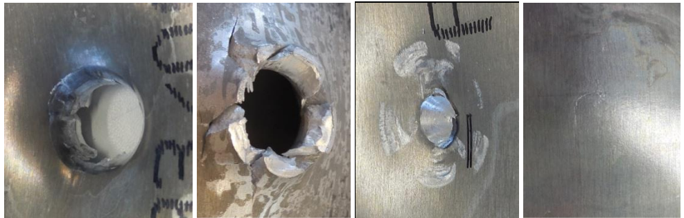
Fig. 2. Test on a multi-layered protection system at 226 m/s. From left to right: front face of the front plate, rear face of the front plate, front face of the rear plate, rear face of the rear plate.
