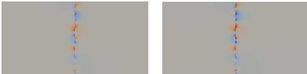
FIGURE 9. Error \mathbf{u}_{\mathcal{T}}^{10} - \mathbf{u}_{\mathcal{T}} at the 10th iteration. Left: primal mesh, \|\mathbf{u}_{\mathcal{M}}^2 - \mathbf{u}_{\mathcal{M}}\|_{\infty} = 0.52 . Right: dual mesh, \|\mathbf{u}_{\mathcal{M}^* \cup \partial \mathcal{M}^*}^2 - \mathbf{u}_{\mathcal{M}^* \cup \partial \mathcal{M}^*}\|_{\infty} = 0.05 .
