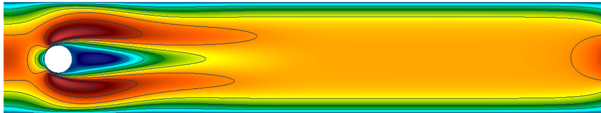
FIGURE 20. First component of the velocity solution to the Navier–Stokes problem on \Omega , obtained at the 559th iteration of the Schwarz algorithm, at T = 2 s.
