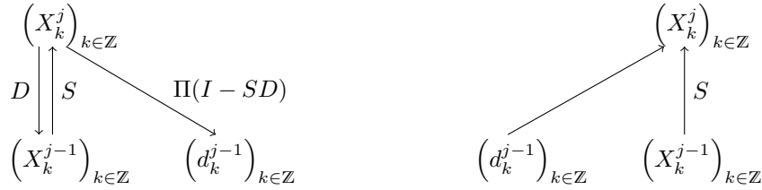
Figure 3: For a given j \in \mathbb{Z} , one scale decomposition (left) and reconstruction (right) with X^j = SX^{j-1} + e^j and d^{j-1} = \Pi e^j .
