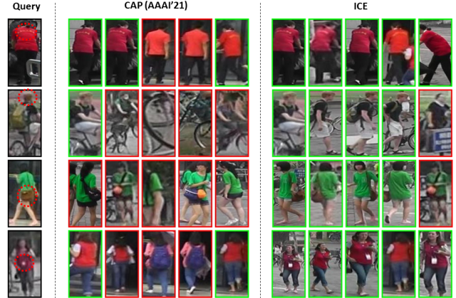
Figure 9: Comparison of top 5 retrieved images on Market1501 between CAP [34] and ICE. Green boxes denote correct results, while red boxes denote false results. Important visual clues are marked with red dashes.
