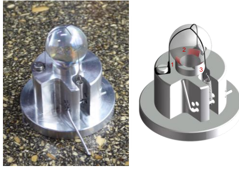
Fig. 3. The retroreflecting sphere and its in-house fastening system. On the left, a photograph of the developed target, and on the right, the 3D model with the feet of the holder in red.
