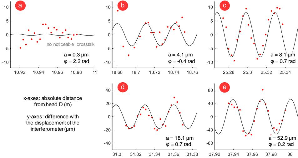
Fig. 17. Difference between the interferometer and the ADM for small displacements.
