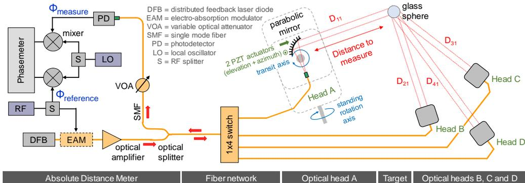
Fig. 1. Functional diagram of the multilateration system.
