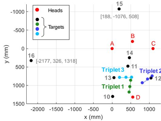
Fig. 18. Top view of the layout of the 4 measurement heads and 16 target positions.
