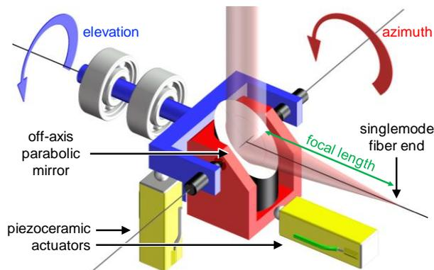
Fig. 2. The second stage of the gimbal mechanism.
