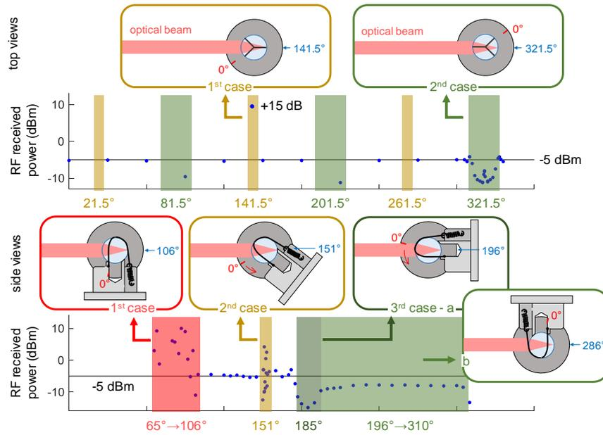
Fig. 10. Impact of the harness: received power when the sphere is rotated around its vertical axis (at the top) and its horizontal axis (at the bottom).
