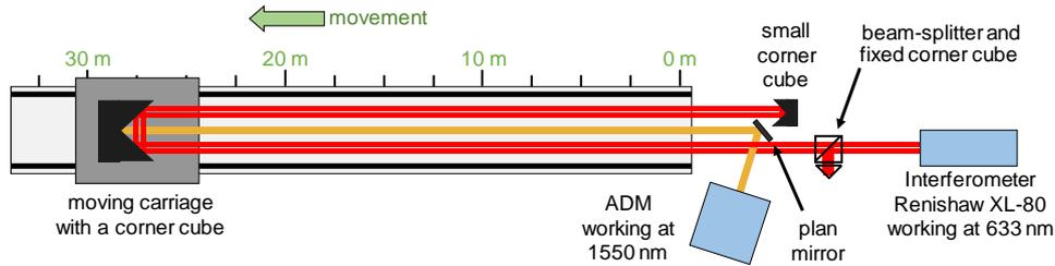
Fig. 13. Comparison between an interferometer and the ADM using a corner cube as target.
