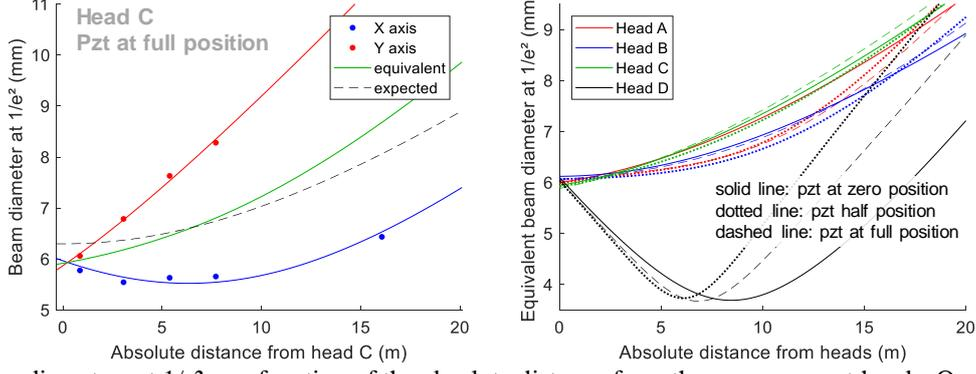
Fig. 8. Beam diameters at  $1/e^2$  as a function of the absolute distance from the measurement heads. On the left: beam diameters of the head C on both axes X and Y. On the right: equivalent beam diameters for the four measurement heads and for different positions of their piezoceramic actuators.
