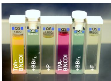
Fig. 9 Absorption spectra of TPA-BNCDI / Tph-BNCDI and their interaction with \text{BBr}_3 and TBAF.
