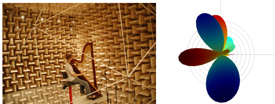
Figure 1: Radiation data recorded in the anechoic chamber of TU Berlin (from [5]) visualized with spat5.hoa.plot.
