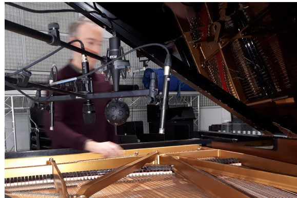
Figure 2: Recording prepared piano with mh acoustics EM32, Sennheiser AMBEO VR, and DPA 4006 omni microphones.
