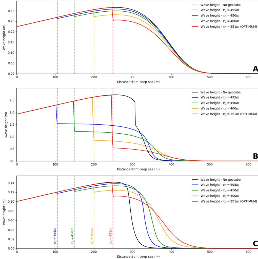
Figure 4: Wave height over the cross-shore profile associated with four geotube positions:  $x_G = 495 m$  (blue),  $x_G = 450 m$  (green),  $x_G = 400 m$  (yellow), and  $x_G = 351 m$  (red). Wave height relating to a seabed profile devoid of geotubes has also been given as a reference (black). **A.** Wave height prior to the storm at  $t = 2$  days. **B.** Wave height at the apex of the storm at  $t = 8.3$  days. **C.** Wave height posterior to the storm at  $t = 18.7$  days.
