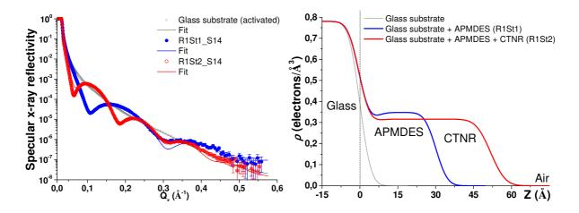
**Figure 2**. **Up**) Specular X-ray reflectivity (XRR) data with best fits to the data (solid lines) of a prefunctionalized glass substrate with APMDES (di-aminosilanes), before and after reaction with CTNR oligomers (respectively in plain blue and empty red marks). **Bottom** Electronic density depth profiles corresponding to the best fit to the XRR data (same color code, see text for experimental conditions).
