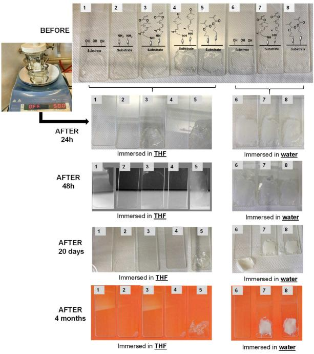
Surface obtained after polymerization with the mixture (F1) before immersed in water/THF
