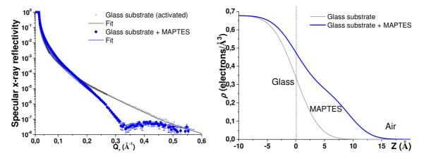
**Figure 4. Left**) Specular X-ray reflectivity (XRR) data with best fits to the data (solid lines) of a prefunctionalized glass substrate with MAPTES. **Right**) Electronic density depth profiles corresponding to the best fit to the XRR data (same color code, see text for experimental conditions).
