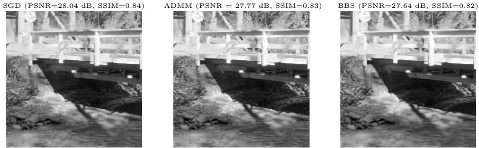
Fig. 7 Plug & Play deblurring, for a 9 \times 9 kernel, an additive Gaussian noise of standard deviation \sigma^2 = (1/255)^2 , for \varepsilon = (5/255)^2 and for the nearly optimal value of \alpha = 0.3 .
