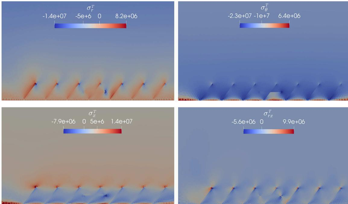
FIGURE 13. *Top*: zoom on the radial and orthoradial total stresses  $\sigma_r^T$  and  $\sigma_\theta^T$  (Pa) at final time for the discontinuous pressure model. *Bottom*: zoom on the axial and shear total stresses  $\sigma_x^T$  and  $\sigma_{rx}^T$  (Pa) at final time for the discontinuous pressure model.
