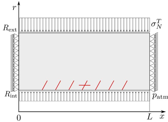
FIGURE 8. Diametral section (not scaled) of the cylinder, with mechanical boundary conditions: zero normal displacement on the two sides  $x = 0$  et  $x = L$  and uniform pressures  $\sigma_N^T$  on the surface  $r = R_{ext}$  and  $p_{atm}$  on the surface  $r = R_{int}$ . The fracture network is highlighted in red.
