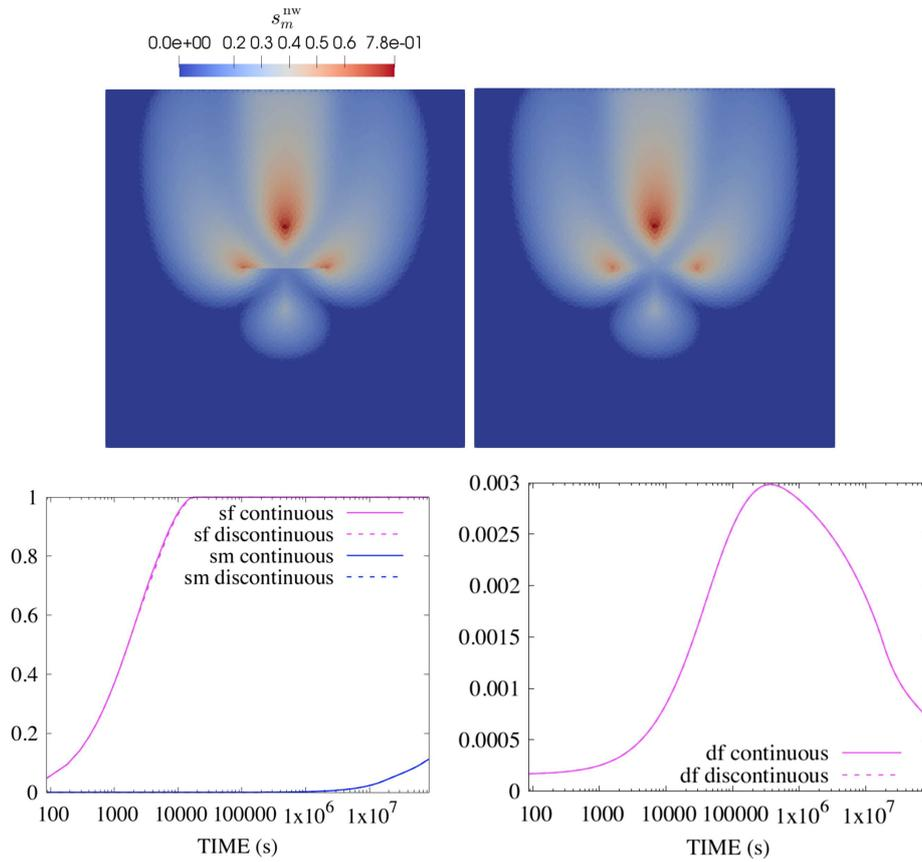
FIGURE 5. *Top*: matrix non-wetting phase saturation at final time obtained by the discontinuous pressure (*left*) and continuous pressure (*right*) models. *Bottom left*: mean non-wetting phase saturations in the matrix and in the fracture network as a function of time for both the continuous and discontinuous pressure models. *Bottom right*: mean fracture apertures ( $m$ ) as a function of time for both the continuous and discontinuous pressure models.
