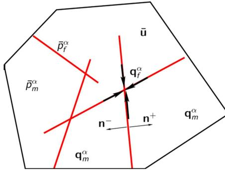
FIGURE 2. Example of a 2D domain  $\Omega$  with its fracture network  $\Gamma$ , the unit normal vectors  $\mathbf{n}^\pm$  to  $\Gamma$ , the phase pressures  $\bar{p}_m^\alpha$  in the matrix and  $\bar{p}_f^\alpha$  in the fracture network, the displacement vector field  $\bar{\mathbf{u}}$ , the matrix Darcy velocities  $\mathbf{q}_m^\alpha$  and the fracture tangential Darcy velocities  $\mathbf{q}_f^\alpha$  integrated along the fracture width.
