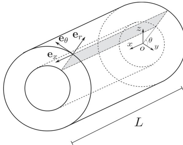
FIGURE 7. Hollow cylinder of length  $L$  and internal and external radii  $R_{\text{int}}$  and  $R_{\text{ext}}$ , respectively. The diametral section is highlighted in gray, the fracture network is not shown for simplicity.
