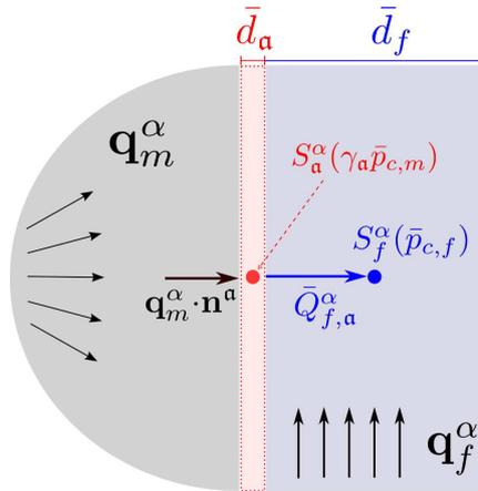
FIGURE 3. Illustration of the flux transmission condition between matrix and fracture, including a layer of damaged rock of thickness  $d_a$ ,  $\mathbf{a} = \pm$ . It can be seen as an upwind two-point-like approximation of  $\bar{Q}_{f,a}^\alpha$ . The arrows show the positive orientation of the normal fluxes  $\mathbf{q}_m^\alpha \cdot \mathbf{n}^a$  (inward with respect to the damaged layer) and  $\bar{Q}_{f,a}^\alpha$  (outward with respect to the damaged layer).
