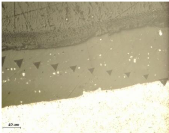
Fig. 13 Imprints on the oxide layer and on the interface
