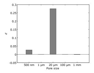
Figure 12. Estimation of the pore size distribution of the CEM I using the serial-parallel model.
