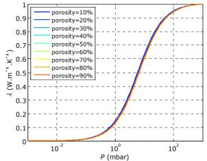
Figure 5. Normalized conductivity as a function of pressure for different porosity rates.
