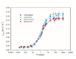
Figure 9. Measured and estimated thermal conductivity versus pressure for each composite.
