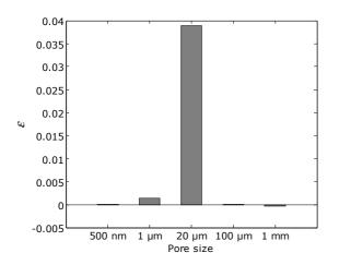
Figure 11. Estimation of the pore size distribution of the UHPC using the serial-parallel model.
