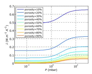
Figure 4. Variation of the thermal conductivity of the air as a function of the pressure for different global porosity rates (d =  $10 \mu m$ ).
