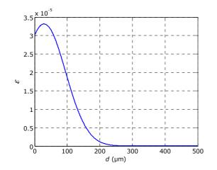
Figure 8. Volume fraction versus normal pore size for the bleached composite from the normal law model.
