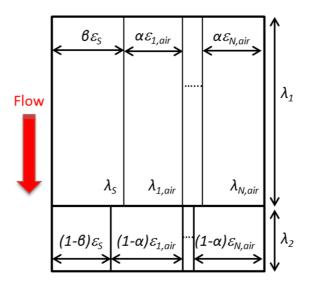
Figure 3. Schematic representation of the serial-parallel model for (N + 1) phases (adapted from [11]).
