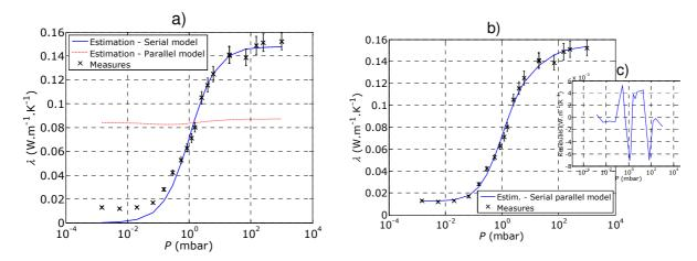
Figure 6. Comparison of the measured and estimated thermal conductivities of the bleached composite
