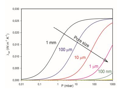
Figure 2. Thermal conductivity of the air as a function of pressure for different pore sizes (at 300 K).
