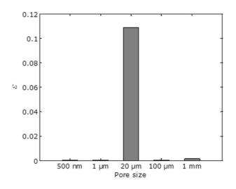
Figure 7. Estimation of the pore size distribution from the serial-parallel model.
