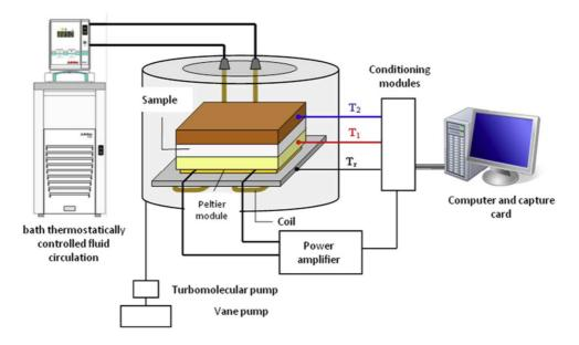
Figure 1. Block diagram of the "DICO" experimental setup [23].
