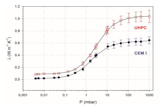
Figure 10. Variation of the thermal conductivity as a function of the pressure of two cement-based materials: CEM I, UHPC. (adjustment with serial/parallel model).
