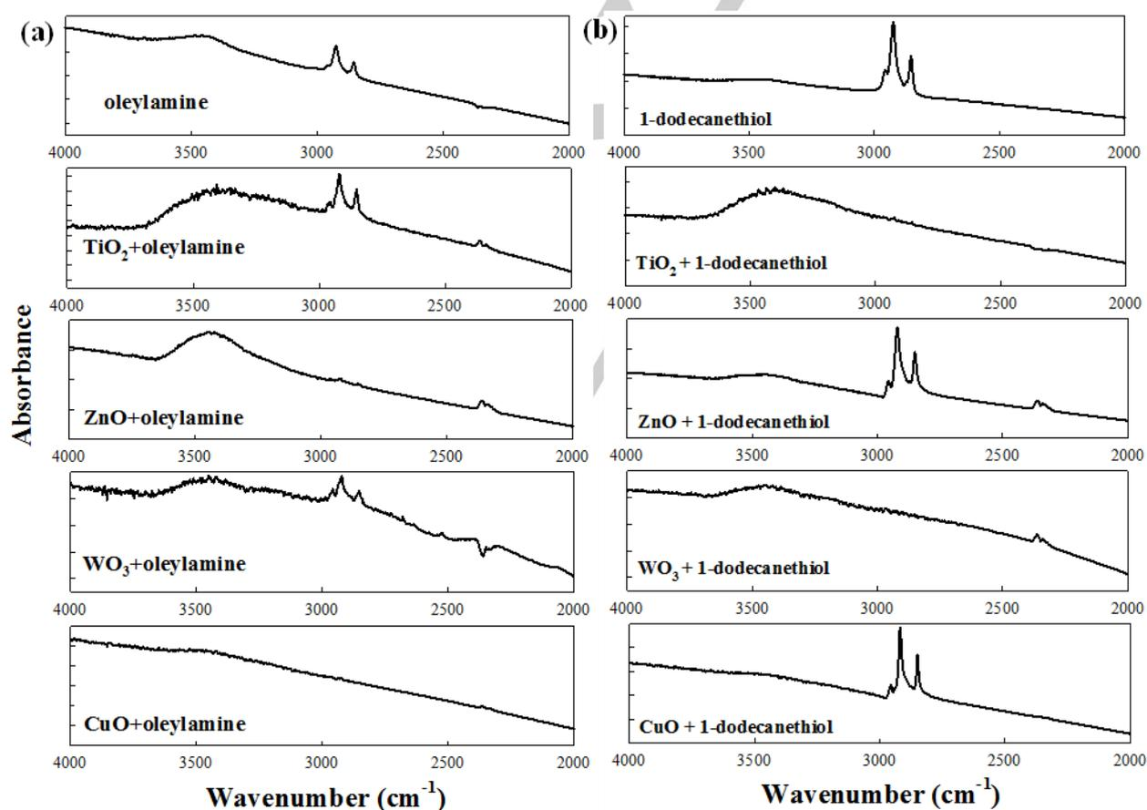
**Figure 1.** FTIR (transmission) spectra comparing  $\nu_s(-\text{CH}_2-)$ ,  $\nu_{as}(-\text{CH}_2-)$ , and  $\nu_{as}(-\text{CH}_3)$  stretches of the alkyl chain of ligand functionalized nanoparticles after four washing cycles: (a) oleylamine and oleylamine + nanoparticles (b) 1-dodecanethiol and 1-dodecanethiol + nanoparticles.
