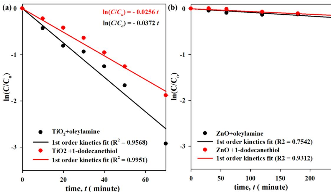
**Figure 6.** Degradation curves of oleylamine and 1-dodecanethiol on (a) TiO<sub>2</sub> and (b) ZnO films respectively fitted to a first order kinetic model. The relative concentrations are estimated from the area of the  $\nu_s(-CH_2-)$ ,  $\nu_{as}(-CH_2-)$ , and  $\nu_{as}(-CH_3)$  bands in the 2800-3000 cm<sup>-1</sup> region.
