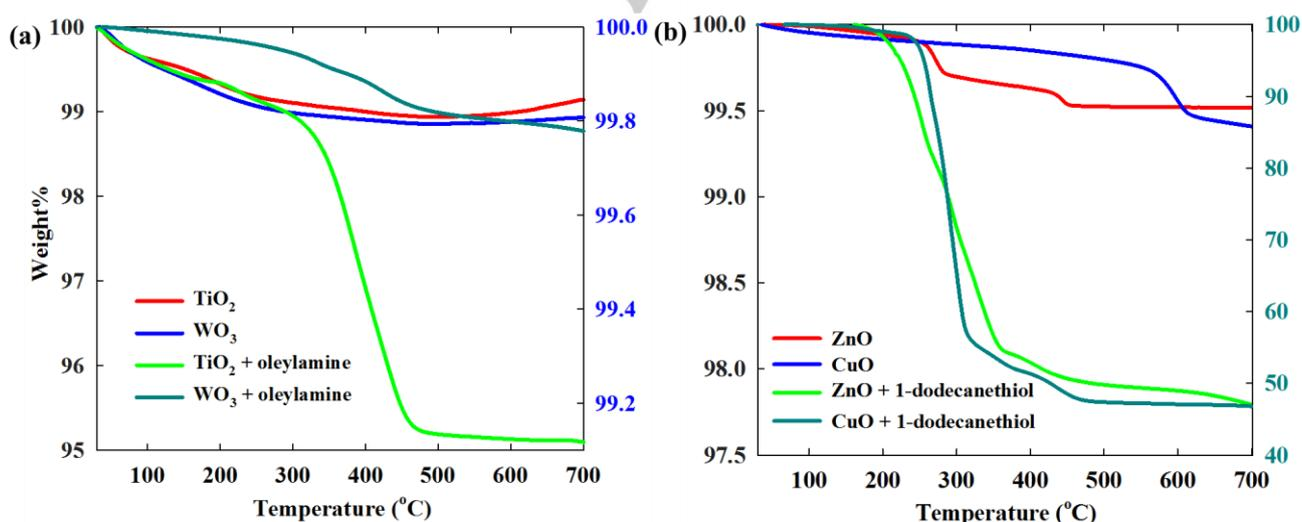
**Figure 4.** Thermogravimetric analysis (TGA) of (a) oleylamine functionalized nanoparticles (b) 1-dodecanethiol functionalized nanoparticles. Right y-axis in Figure (a): WO<sub>3</sub> powder, right y-axis in Figure (b): CuO + 1-dodecanethiol
