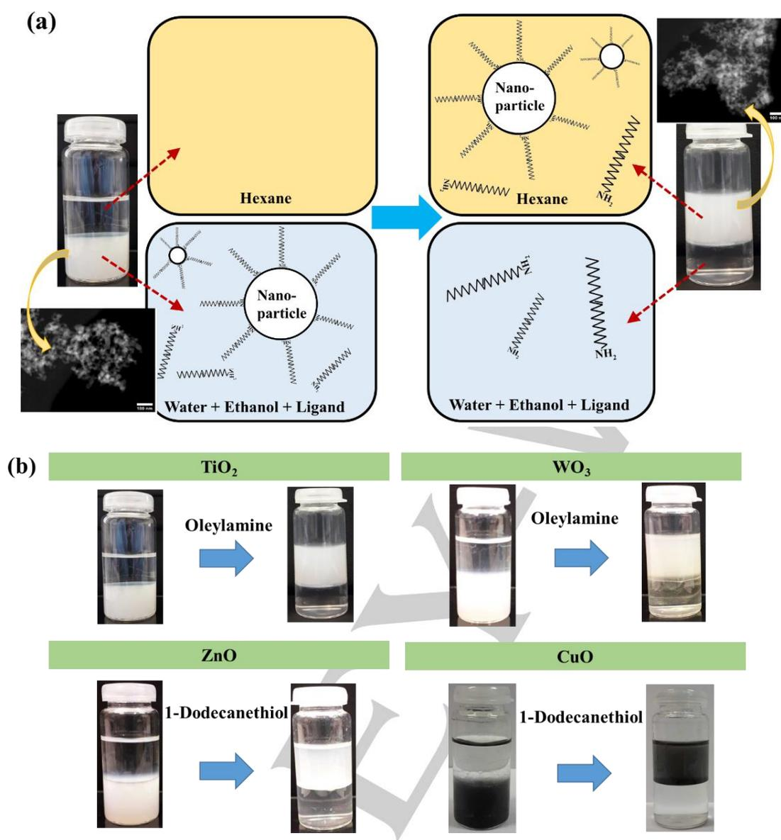
**Figure 2.** (a) Schematic explanation of the polar to non-polar phase transfer procedure of nanoparticles (inset: HAADF-STEM images of  $\text{TiO}_2$  nanoparticles before and after phase transfer with 100 nm scale bar). (b) Successful phase transfer of each nanoparticle with its specific ligand.
