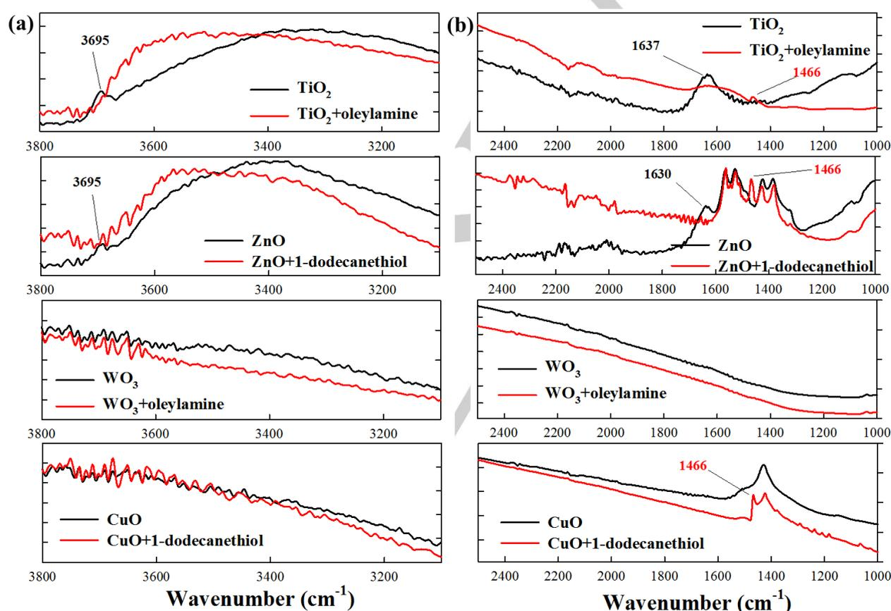
**Figure 3.** ATR-FTIR spectra of ligand functionalized nanoparticles (red) compared with their pure powders (black) in the (a)  $3800\text{--}3100\text{ cm}^{-1}$  (b)  $2500\text{--}1000\text{ cm}^{-1}$  regions in terms of  $\text{H}_2\text{O}$  adsorption bands.
