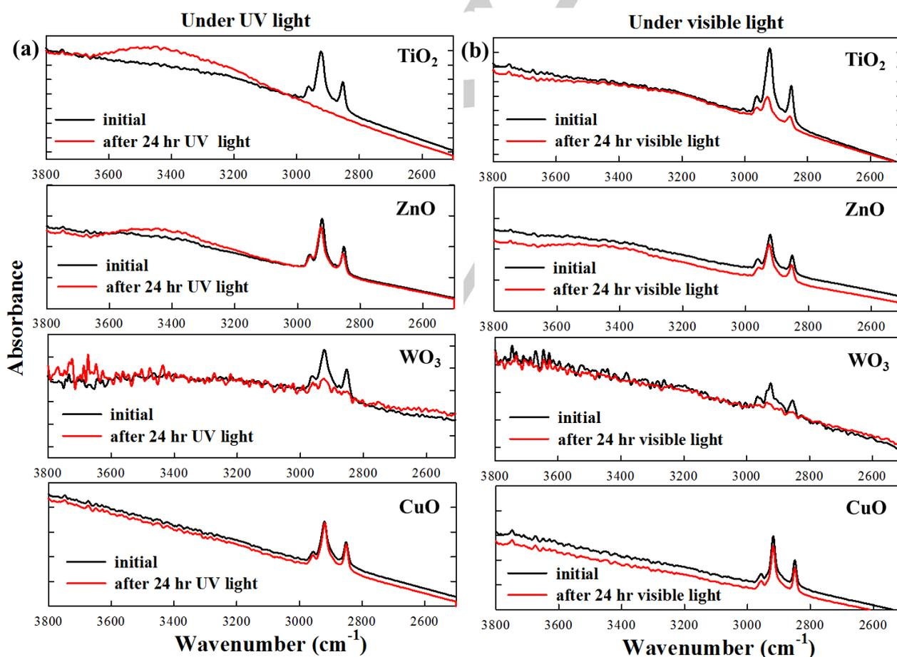
**Figure 5.** FTIR spectra ( $\nu_s(-CH_2-)$ ,  $\nu_{as}(-CH_2-)$ , and  $\nu_{as}(-CH_3)$  bands in the 2800-3000  $cm^{-1}$  region) of ligand capped nanoparticle films on a Si substrate showing photo-stability of the ligands on the nanoparticles under (a) UV (b) visible light.
