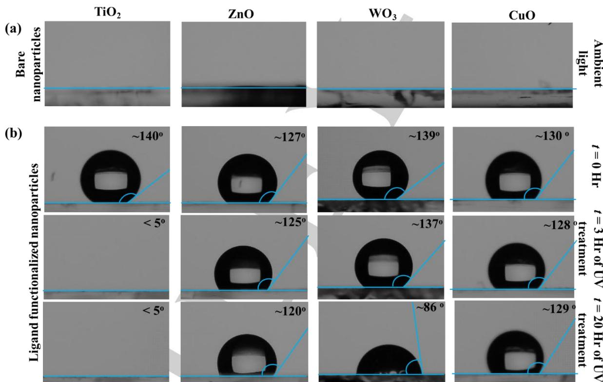
**Figure 7.** Water contact angle on drop-casted ligand capped nanoparticle films: (a) ligand free bare nanoparticles (b) hydrophobic functionalized nanoparticles, also showing the effect of UV irradiation. The contact angles are average of five measurements and the blue lines marking the angles are for representation.
