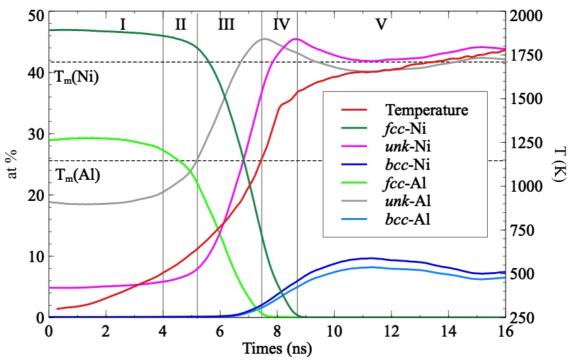
Figure 4. Temperature profile and structure analysis in a slice of 40 nm, around x = 150 nm.
