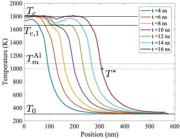
Figure 2. Temperature profiles. The horizontal lines indicate:  $T_0$ , the initial temperature;  $T_m^{\rm Al}$ , the melting temperature of A;  $T_c$ , the combustion temperature at 12 ns. The dot indicates  $T^*$ , the reference temperature corresponding to the instantaneous position of the front.
