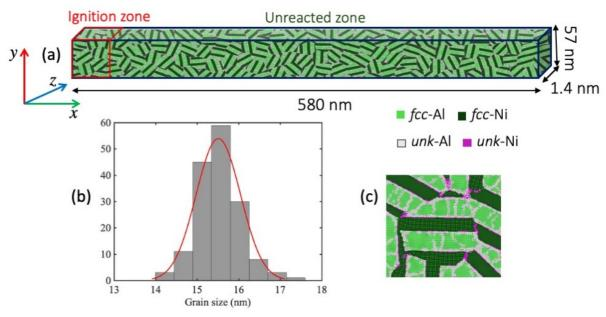
Figure 1. (a) Schematic representation of the initial state of the system. (b) Histogram of average grain sizes. (c) Enlarged view of a lamellar grain.
