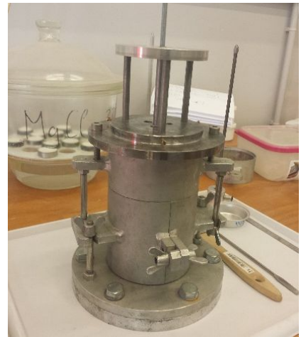
Figure 5. (a) Geometry and (b) picture of the split standard Proctor mould used for experimental testing.
