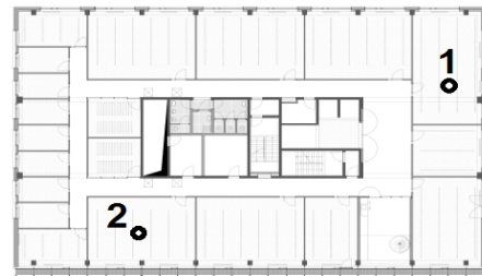
Figure 4. Ground plan of office building used for measurements. The circles show the location of the measurements.
