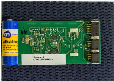
Figure 2. An example of an LTE 2600 node including a textile antenna and a PCB.
