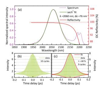
**Fig. 3.** Optical spectrum (a) of the mode-locked Tm:LuYO<sub>3</sub> ceramic laser with  $T_{OC} = 0.5\%$ , and the corresponding interferometric autocorrelation traces before (b) and after (c) compression. The red curve in (a) shows the reflectivity of the output coupler.
