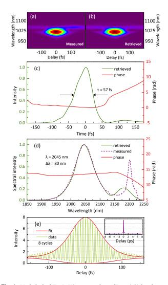
**Fig. 4.** Mode-locked Tm:LuYO<sub>3</sub> ceramic laser ( $T_{OC} = 0.5\%$ ) – shortest pulses. Measured (a) and retrieved (b) SHG-FROG traces after external pulse compression using ZnS, and the reconstructed temporal (c) and spectral (d) intensity and phase profiles; the dashed line in (d) is the measured optical spectrum. (e) interferometric autocorrelation trace. Inset (e): corresponding noncollinear autocorrelation trace on a time scale of ±7.5 ps.
