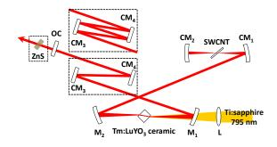
**Fig. 1.** Schematic of the SWCNT-SA mode-locked Tm:LuYO<sub>3</sub> ceramic laser. (L, lens; M<sub>1</sub>-M<sub>2</sub>, dichroic mirrors; CM<sub>1</sub>-CM<sub>4</sub>, chirped mirrors; OC, output coupler).
