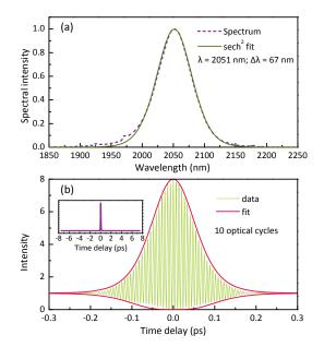
Fig. 2. Mode-locked Tm:LuYO<sub>3</sub> ceramic laser ( $T_{0C} = 3\%$ ). Optical spectrum (a) and interferometric autocorrelation trace (b). Inset (b): corresponding noncollinear autocorrelation trace on a time scale of  $\pm 7.5$  ps.
