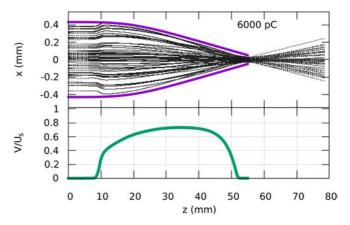
FIG. 3. Ion trajectories (black) after 6000 pC have been injected. Configuration GND was used and the profile of the inner surface of the capillary are shown in violet. Below we show the electric potential normalized with respect to the potential of the ion source  $U_s$
