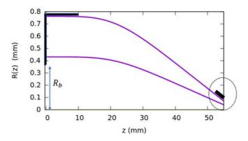
FIG. 1. Profile of the inner and outer glass-vacuum interfaces of the capillary. Black solid lines stand for the grounded conducting electrodes.  $R_b = 0.4$  mm is the radius of the hole in the grounded collimator plate in front of the capillary. Setup INS and GND differ by the 3 mm short grounded electrode that covers the tip (circled) and which is absent in setup INS.
