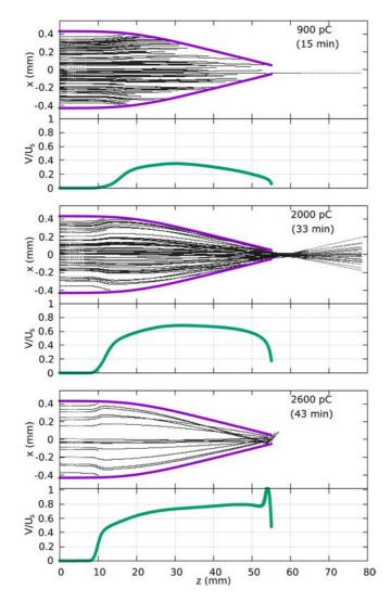
FIG. 2. Ion trajectories (black) at three different moments, identified by the injected charge Q or in brackets by the injection time  $(Q/I_{\rm in})$ . Beam intensity is  $I_{\rm in}=1$  pA. Configuration INS was used and the profile of the inner surface of the capillary are shown in violet. Below each panel showing the trajectories, the electric potential, normalized with respect to the potential of the ion source  $U_s$ , is given.
