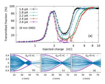
FIG. 5. (a) Evolution of the transmitted fraction as a function of the injected charge Q for various beam intensities  $I_{\rm in} \in [1.6, 2.6] \, \rm pA$ . Configuration GND is used but with a grounded tip electrode which is 8 mm long. (b), (c) and (d) show the trajectories at different moments indicated by the injected charge  $Q_{\rm in}$ , for the case  $I_{\rm in} = 2.4 \, \rm pA$ .
