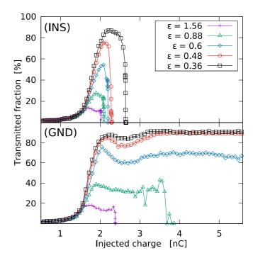
FIG. 7. Evolution of the transmitted fraction as a function of the injected charge for various emittances  $\epsilon \equiv \epsilon_{rms} \in [0.3, 1.6]$  mmm rad. The chosen configuration is shown in the top left corner. Intensity of the injected current was 1 pA.
