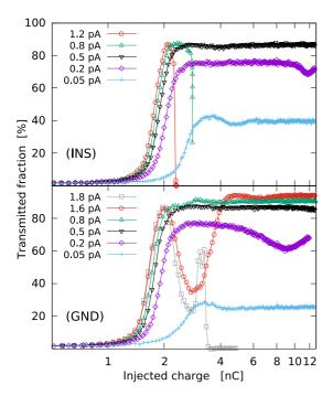
FIG. 4. Evolution of the transmitted fraction as a function of the injected charge for various beam intensities  $I_{\rm in} \in [0.05, 1.8]\, \rm pA$ . Injected beam emittance was  $\epsilon_{\rm rms} = 0.36\, \rm mm$  mrad. Top panel used configuration INS and bottom panel configuration GND. Note the x-log scale.
