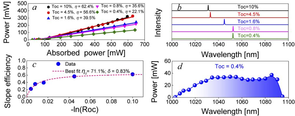
**Fig. 3.** CW laser performance of the Yb:GdYCOB crystal for different OCs (a); measured laser spectra in the CW regime (b), slope efficiency as a function of the OC reflectivity  $1 - T_{OC}$  (c), and spectral tuning obtained with a SF10 prism in the CW regime for  $T_{OC} = 0.4\%$  (d).
