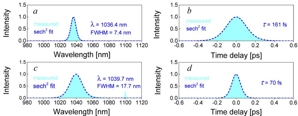
**Fig. 4.** Characterization of the transition of the ML Yb:GdYCOB laser from SESAM ML to KLM with  $T_{oc} = 4.5\%$ . ML optical spectra with  $\text{sech}^2$  fit indicating soliton pulses: (a) SESAM ML and (c) KLM; autocorrelation traces with  $\text{sech}^2$  fit: (b) SESAM ML and (d) KLM.
