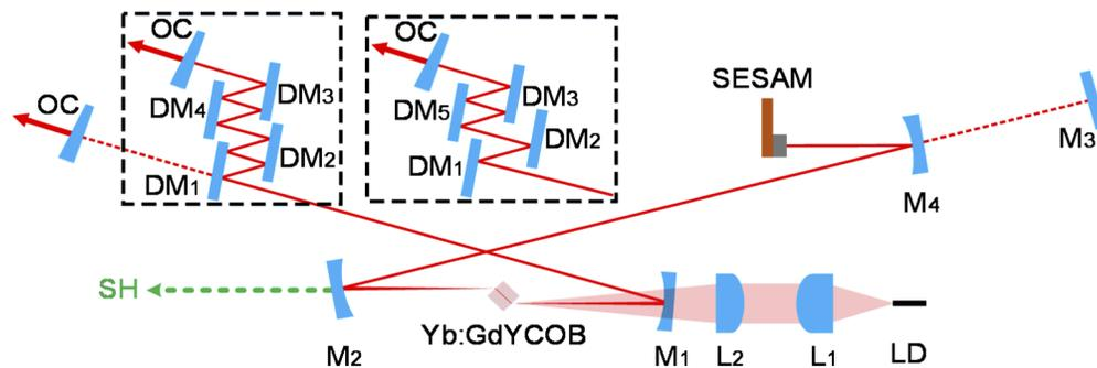
**Fig. 2.** Experimental arrangement of the CW and KLM Yb:GdYCOB laser. LD: fiber-coupled laser diode; L<sub>1</sub>: collimating aspherical lens; L<sub>2</sub>: focusing achromatic doublet; M<sub>1</sub>-M<sub>2</sub>: concave dichroic mirrors; M<sub>3</sub>: flat rear mirror in CW operation; DM<sub>1</sub>-DM<sub>5</sub>: dispersive mirrors; OC: output coupler; SH: second-harmonic output.
