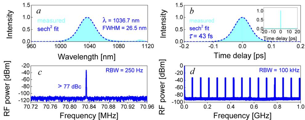
**Fig. 6.** Measured ML spectrum of the Yb:GdYCOB laser with  $T_{\text{OC}} = 2.5\%$  (a) and intensity autocorrelation trace with a  $\text{sech}^2$ -fit (b). Inset: autocorrelation trace in the time span of 40 ps; RF spectra of the ML Yb:GdYCOB laser: fundamental beat note (c) and 1-GHz span (d).
