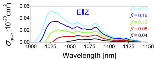
**Fig. 1.** Gain cross-section spectra,  $\sigma_{\text{gain}}$ , for Yb<sup>3+</sup> ions in the “mixed” Yb:GdYCOB crystal for light polarization *E* || *Z*,  $\beta$  is the inversion ratio.
