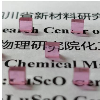
**Fig. 1.** Photograph of annealed and polished Er:(Lu,Sc)<sub>2</sub>O<sub>3</sub> ceramic elements.
