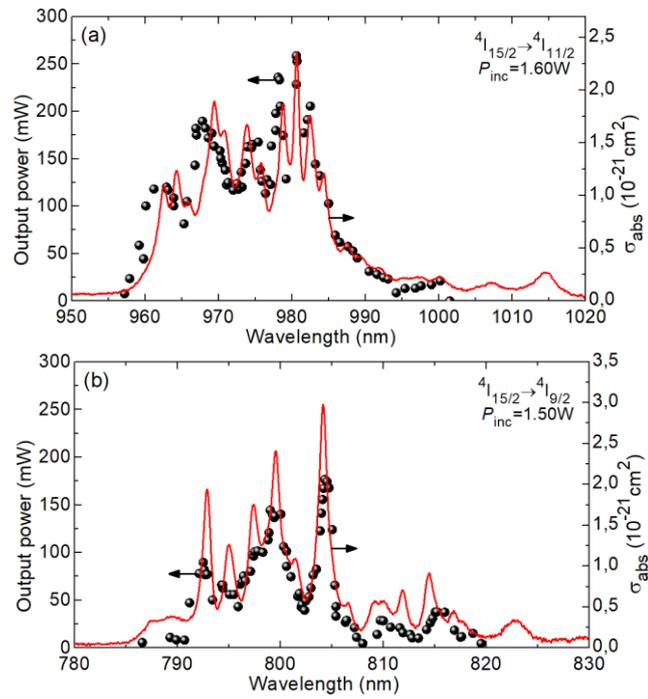
**Fig. 12.** Laser excitation curves for the Er:(Lu,Sc)<sub>2</sub>O<sub>3</sub> ceramic laser (output power vs. the pump wavelength) measured at a fixed incident pump power  $P_{inc}$ : pumping into (a) the  $^4I_{15/2}$  state and (b) the  $^4I_{9/2}$  state. Symbols – laser output power, curves –  $\sigma_{abs}$  spectra.
