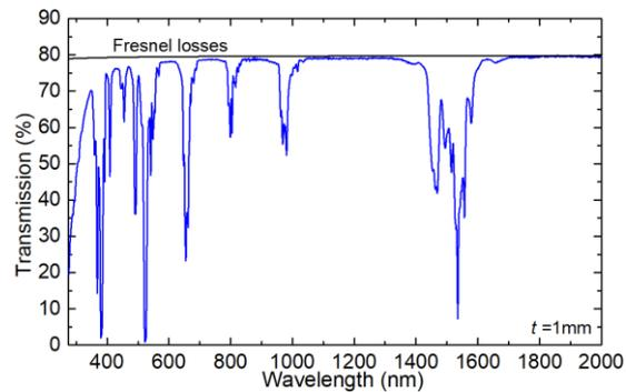
**Fig. 4.** Transmission spectrum of a laser-grade-polished Er:(Lu,Sc)<sub>2</sub>O<sub>3</sub> ceramic disk (thickness,  $t = 1.0 \text{ mm}$ ), black curve – theoretical transmission determined by the Fresnel losses.
