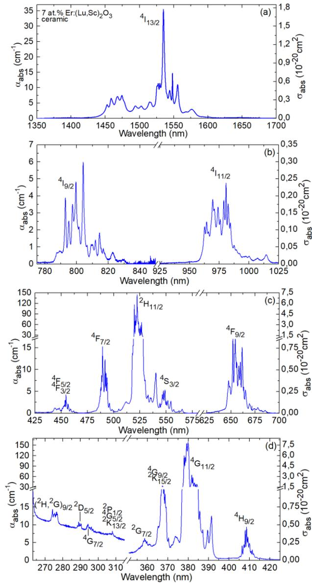
**Fig. 5.** (a-d) RT absorption spectra of 7 at.% Er:(Lu,Sc)<sub>2</sub>O<sub>3</sub> ceramic ( $\alpha_{\text{abs}}$  – absorption coefficient,  $\sigma_{\text{abs}} = \alpha_{\text{abs}}/N_{\text{Er}}$  – absorption cross-section).
