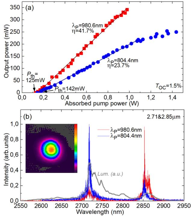
**Fig. 11.**  $\text{Er}:(\text{Lu},\text{Sc})_2\text{O}_3$  ceramic laser: (a) input-output power dependences for  $\lambda_P = 804.4$  nm and 980.6 nm,  $\eta$  – slope efficiency; (b) typical laser emission spectra, *inset* – spatial profile of the laser mode in the far-field.  $T_{OC} = 1.5\%$ . The laser emission is unpolarized. For comparison the luminescence curve is implemented (gray).
