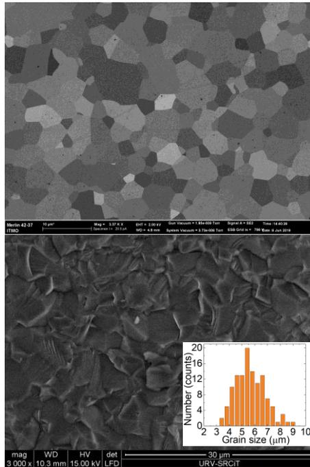
**Fig. 3.** Microstructure of Er:(Lu,Sc)<sub>2</sub>O<sub>3</sub> ceramic: (a) SEM images of the polished surface; (b) environmental SEM image of the fracture surface. Inset in (b) – grain size distribution. Scale
