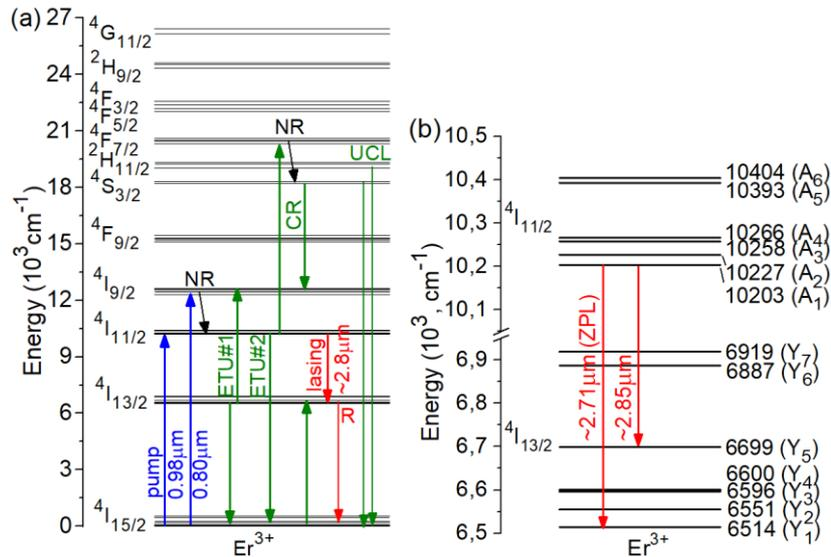
**Fig. 9.** Scheme of energy-levels of Er<sup>3+</sup> ions in C<sub>2</sub> sites in (Lu,Sc)<sub>2</sub>O<sub>3</sub> ceramic: (a) general scheme: *blue and red arrows* – pump and laser transitions, respectively, ETU – energy-transfer upconversion, CR – cross-relaxation, R and NR – radiative and non-radiative transitions, respectively, UCL – upconversion luminescence; (b) splitting of the <sup>4</sup>I<sub>11/2</sub> and <sup>4</sup>I<sub>13/2</sub> multiplets, *arrows* – observed laser lines.
