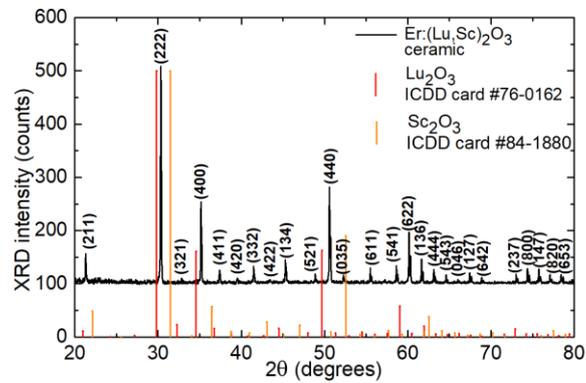
**Fig. 2.** X-ray powder diffraction pattern of Er:(Lu,Sc)<sub>2</sub>O<sub>3</sub> ceramic, *red and orange peaks* – theoretical patterns for Lu<sub>2</sub>O<sub>3</sub> (ICDD card #76-0162) and Sc<sub>2</sub>O<sub>3</sub> (ICDD card #84-1880), respectively, *numbers* – Miller's indices (*hkl*).
