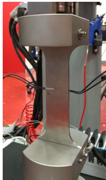
Figure 1. Experimental configuration of a PVR test with two thermocouples.
