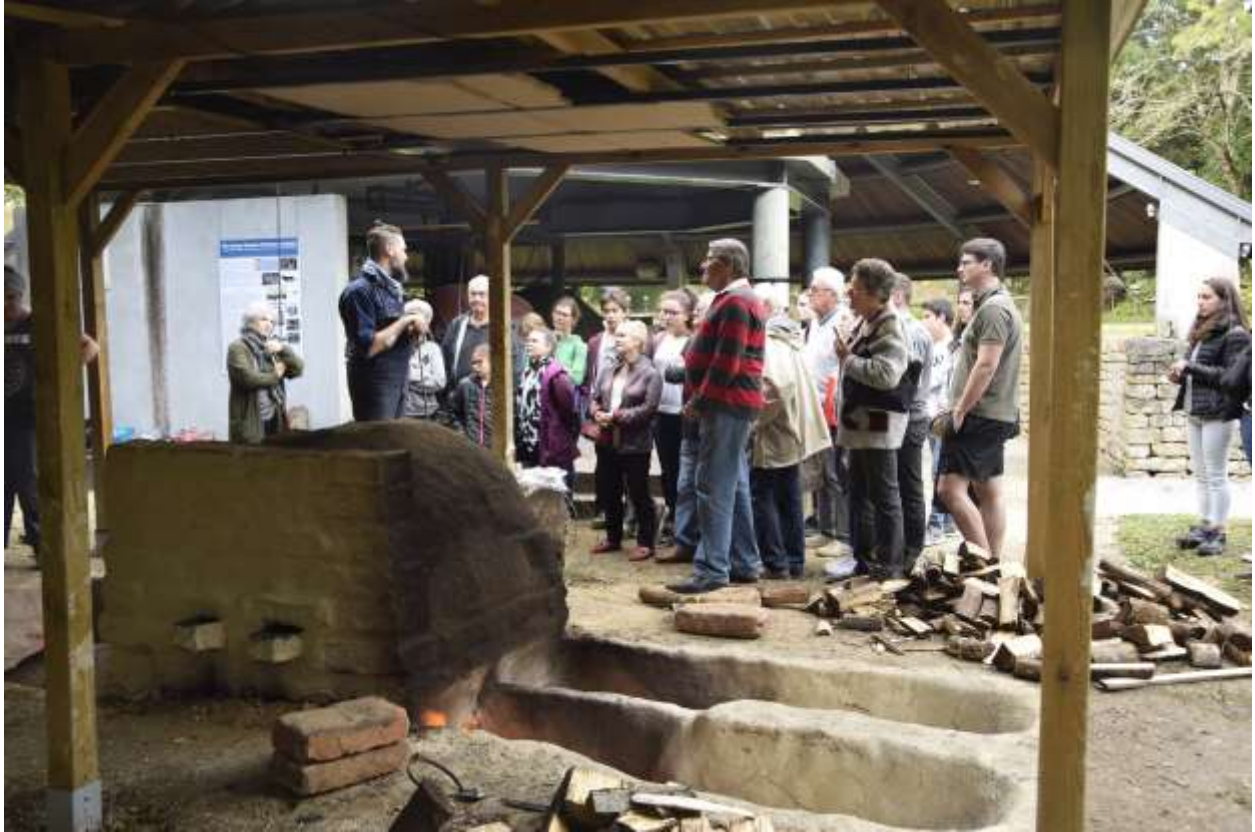
Figure 4: A reconstruction of the Kerma bronze casting furnace by Georges Verly, Frederik Rademakers and colleagues.
