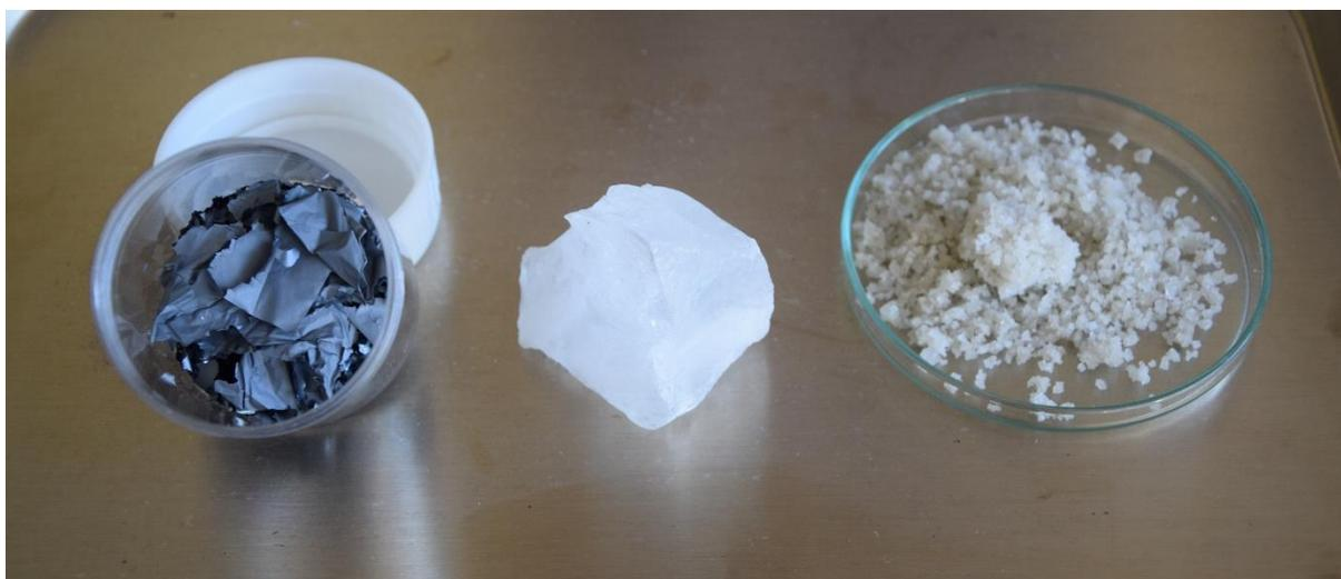
Figure 1. Raw materials, from left to right: copper scale, alum and sea salt.
