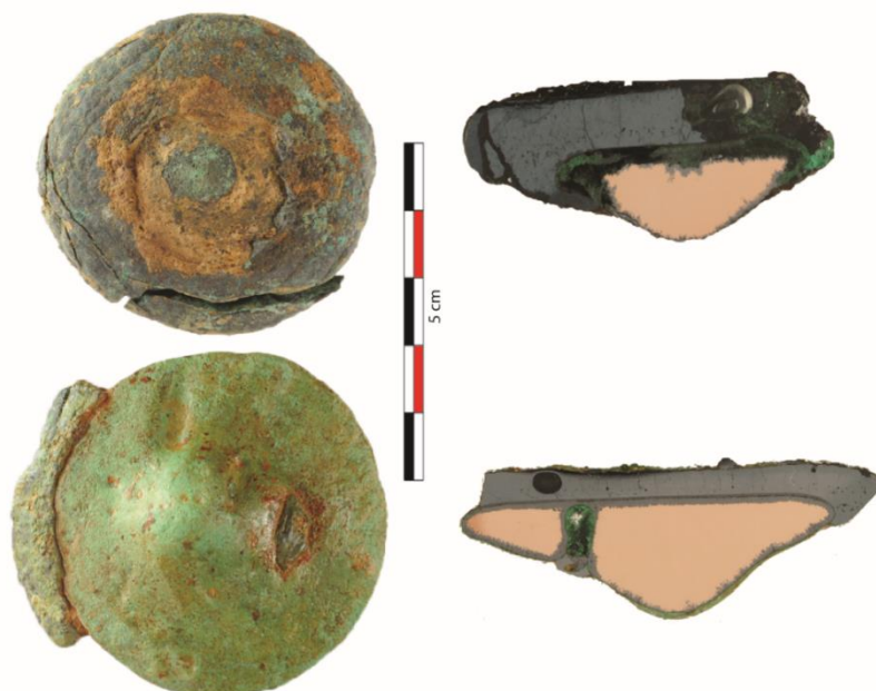
Figure 2: Examples of the intermediate metallic products identified with a matte layer (black layer) covering the metallic copper
