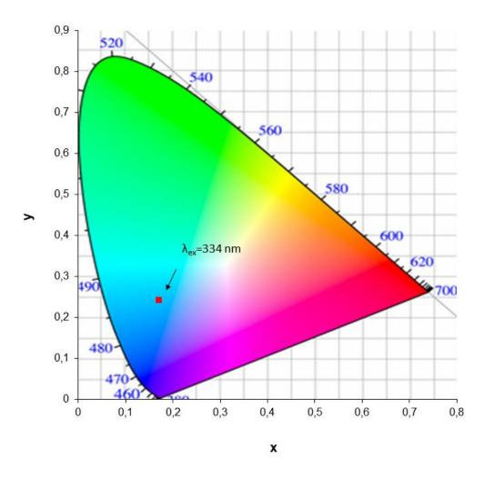
Fig. 7 CIE chromaticity diagram of the compound under an excitation of 334 nm.
