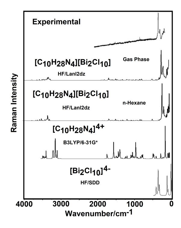
Fig. 9 Raman spectrum of  $(C_{10}H_{28}N_4)[Bi_2Cl_{10}]$  recorded in the solid phase at room temperature compared with the corresponding predicted for cation, anion and compound in gas phase and n-hexane solution by using different methods.
