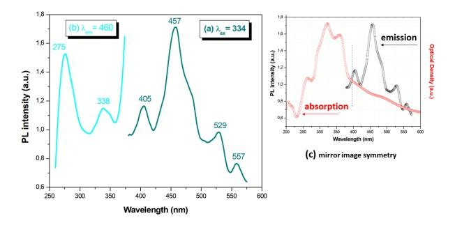
Fig. 6 Solid-state luminescence spectra: emission (a) and excitation (b) of  $(C_{10}H_{28}N_4)[Bi_2Cl_{10}]$ ; mirror image symmetry of the emission and absorption spectra (c).
