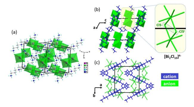
**Fig 2.** (a) Perspective view of (C<sub>10</sub>H<sub>28</sub>N<sub>4</sub>)[Bi<sub>2</sub>Cl<sub>10</sub>]; (b) Geometry of [Bi<sub>2</sub>Cl<sub>10</sub>]<sup>4-</sup> dimer; (c) Orientation of organic molecules (in blue), which occupy the empty spaces among inorganic entities (in green).
