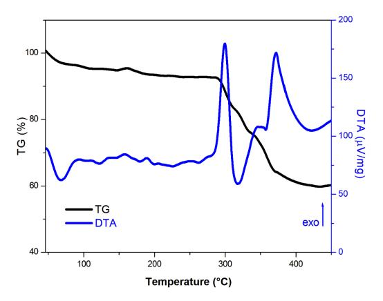
Fig. 10 TG-DTA curve of  $(C_{10}H_{28}N_4)[Bi_2Cl_{10}]$ .
