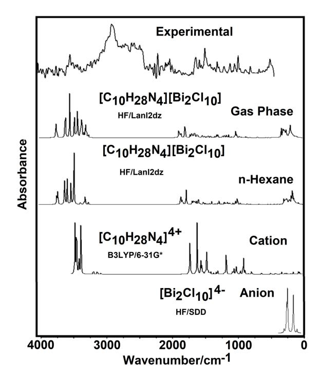
**Fig.8** FTIR spectrum of  $(C_{10}H_{28}N_4)[Bi_2Cl_{10}]$  in the solid phase compared with the corresponding predicted for cation, anion and compound in gas phase and n-hexane solution by using different methods.
