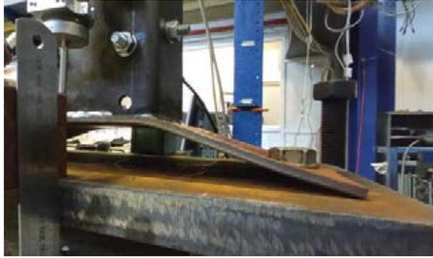
Figure 4: Lateral view of the specimen at the end of the monotonic test
