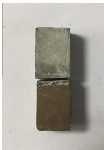
Fig. 3. Composite cracking after the thermal cycle of 80 °C during 3 days.
