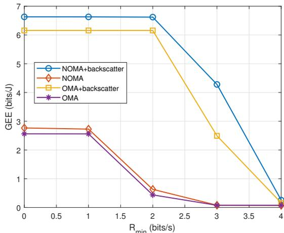
Fig. 4. Energy efficiency as a function of  $R_{\min}$  for  $K = 3$  users and  $P_{\max} = 50$  dBm. Backscatter-aided NOMA outperforms all other schemes. The larger the required QoS, the more power is consumed at the BS, decreasing the energy efficiency.
