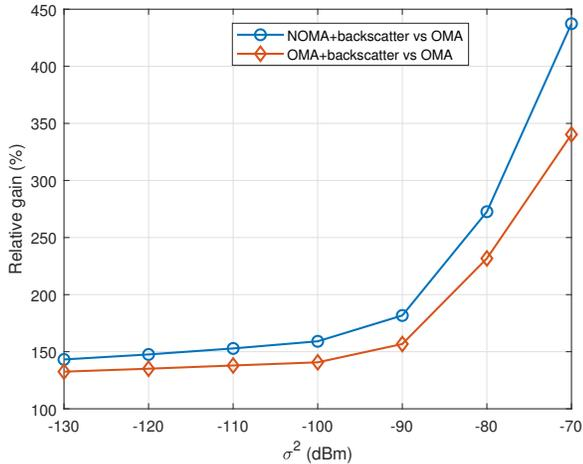
Fig. 3. Relative energy efficiency gain of backscatter-aided NOMA and backscatter-aided OMA compared to conventional OMA as a function of  $\sigma^2$  for  $K = 3$  users,  $R_{\min} = 1$  bits/s and  $P_{\max} = 50$  dBm: the relative gain of NOMA with backscattering goes up to 450%; whereas the one of OMA with backscattering reaches 350%.
