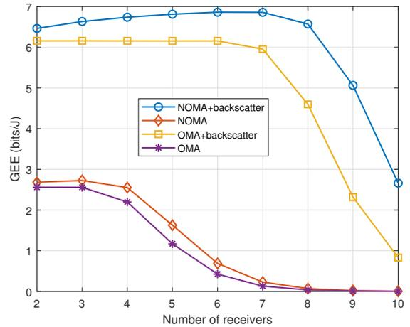
Fig. 1. Energy efficiency ( $GEE$ ) as a function of the number of users  $K$  for  $R_{\min} = 1$  bit/s. Backscattering always improves the energy efficiency of both NOMA and OMA irrespective from the number of users  $K$ . When  $K$  grows large the backscattering advantage decreases.
