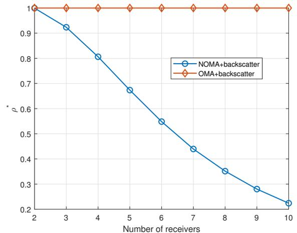
Fig. 2. Optimal reflection coefficient  $\rho^*$  as a function of the number of users  $K$  for  $R_{\min} = 1$  bit/s. For OMA, the ambient incident signal from the BS is completely reflected and  $\rho^* = 1$ , while for NOMA, only a part of the incident signal is reflected ( $\rho^* < 1$ ), the other part being exploited for energy harvesting.
